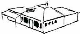
Motel Tearoom/Gift Shop truncated hip roof, lean-to wing, and flat-roofed rear ell.
