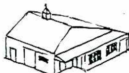
Sign shop Gable roof barn converted to Saltbox style.
